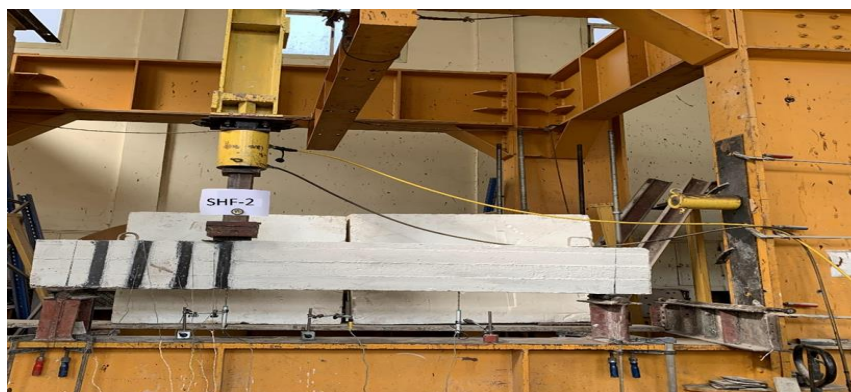
Fig (3): The Casted Beams During Testing
