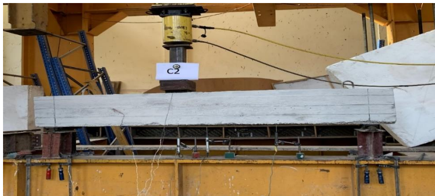
Fig (2): The Control beam During Testing
