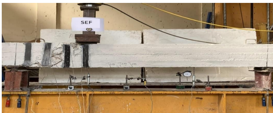
Fig (6): Tested specimen after failure.
