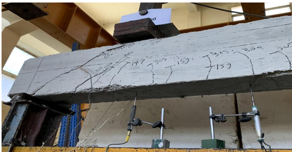
Fig (5): crack pattern during testing of specimen.
